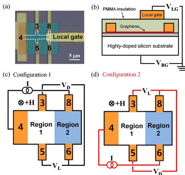
FIG. 1. (Color online) (a) Optical image of the sample. A PMMA insulation layer covers the graphene sheet, the boundary of which is defined by white broken lines. The white scale bar represents  $5 \mu\text{m}$ . (b) Schematic gate configuration. (c) Measurement configuration 1. (d) Measurement configuration 2.
