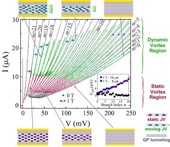
Fig. 2: Detailed  $I$ - $V$  curves in an in-plane field of 1 T (red and green curves) along with the zero-field IQT (grey) curves. Schematic vortex configurations corresponding to a few branches are illustrated. Inset: the voltage difference ( $V_{diff}$ ) between neighboring in-field and zero-field branches for each  $m$  for the given bias currents. The line is a guide to the eyes.
