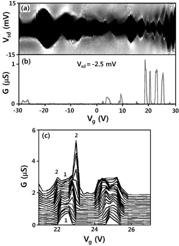
Fig. 3. (a) Gray-scale plot of the differential conductance as a function of  $V_g$  and  $V_{sd}$  at 50 mK. The black and the bright areas are the zero-conductance and the finite-conductance regions, respectively. (b) A part of the gray-scale plot for  $V_{sd} = -2.5$  mV. (c) Conductance *vs*  $V_g$  graph, for different  $V_{sd}$  ranging from  $-2.0$  mV to  $-3.9$  mV in steps of  $-0.1$  mV from bottom to top.
