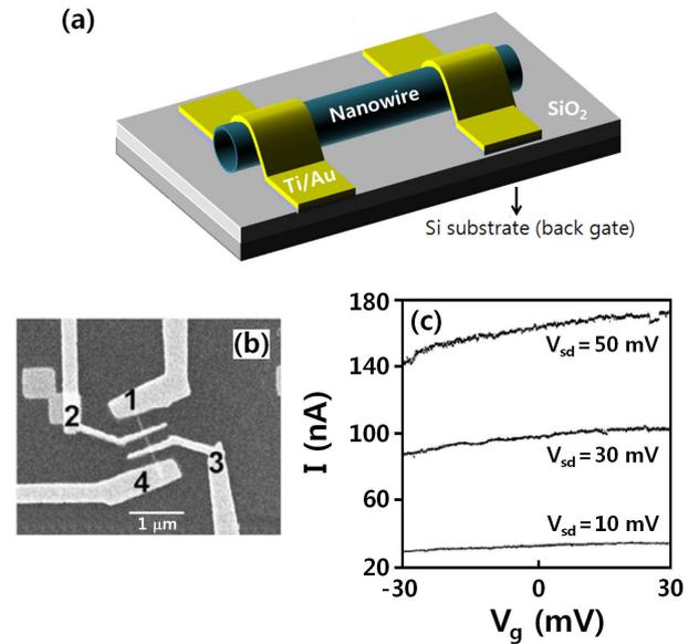
Fig. 1. (a) Schematic configuration of a coaxial  $\text{Zn}_{0.8}\text{Mg}_{0.2}\text{O}/\text{ZnO}$  nanorod device with two Ti/Au Schottky-contact electrodes attached. (b) An SEM image of nanorod B. Two-probe measurements were made using electrodes 2 and 3. (c) Current-voltage curves for source-drain biases of  $V_{sd} = -10, -30$  and  $-50$  mV at room temperature, which show n-type semiconducting characteristics.
