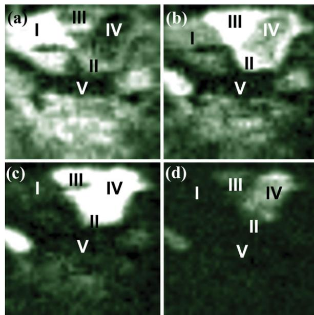
**Figure 2.** SPEM images simultaneously measured at different BE windows of a) 285.2, b) 284.8, c) 284.4, and d) 284 eV. The width of each window is 0.4 eV. It shows specific graphene layers with higher intensity depending on the specific BE window.
