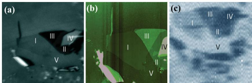
**Figure 1.** a) Optical image of a graphene flake consisting of mono- and multilayer graphene, b) AFM image,  $20 \times 20 \mu\text{m}^2$ , c) SPEM image,  $25 \times 25 \mu\text{m}^2$ . Region I, monolayer graphene; region II, double-layer graphene; region III, triple-layer graphene; region IV, multilayer graphene; region V,  $\text{SiO}_2$  substrate.
