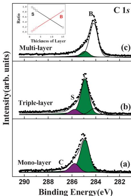
**Figure 3.** Photoemission spectra of C 1s core-level spectra measured on the local regions of I, III, and IV. These were measured at the photon energy of 635 eV (raw data (open circles), solid red lines (fitted data), monolayer components (gray areas), and multilayer components (hatched areas)). The inset shows an area ratio of monolayer component S (open squares) and multilayer component B (open circles) depending on the layer thickness.
